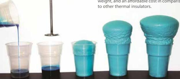
with volumizing agents. In order to achieve a polyurethane foam with the highest thermal insulation, the gas of the pores should have a low thermal conductance.
